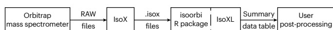
Fig. 3 | Workflow of isotope ratio data processing. The RAW data from the Orbitrap mass spectrometer can be processed by using the following software that has been custom-written for the ESI-Orbitrap IRMS analysis: IsoX software that generates .isox files, which can be processed by using R scripts or functions available in the isoorbi R package or the IsoXL graphical user interface. As a result, a simple summary data table is provided.
